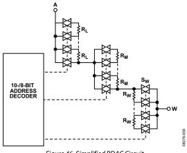
Figure 46. Simplified RDAC Circuit
