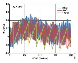
Figure 9. R-INL in R-Perf Mode vs. Code vs. Nominal Resistance (AD5272)
