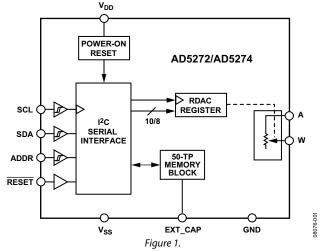
The AD5272/AD5274 device wiper settings are controllable through the I<sup>2</sup>C-compatible digital interface. Unlimited adjustments are allowed before programming the resistance value into the 50-TP memory. The AD5272/AD5274 do not require any external voltage supply to facilitate fuse blow and there are 50 opportunities for permanent programming. During 50-TP activation, a permanent blow fuse command freezes the wiper position (analogous to placing epoxy on a mechanical trimmer).
