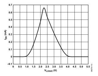
Figure 23. Supply Current (IDD) vs. Digital Input Voltage
