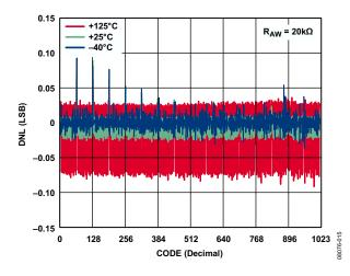
Figure 12. R-DNL in Normal Mode vs. Code vs. Temperature (AD5272)
